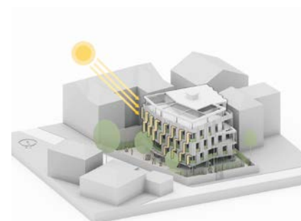
Sun protection. Additional sun protection without hiding views with Fabric facade
